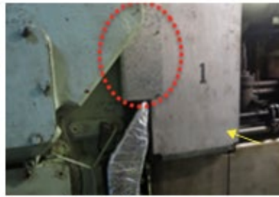
Shielding to protect the turbocharger
