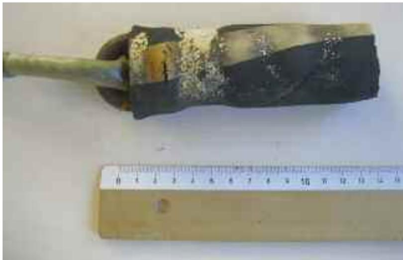
A steel bar used as a weight, covered by a piece of reinforced hose.
