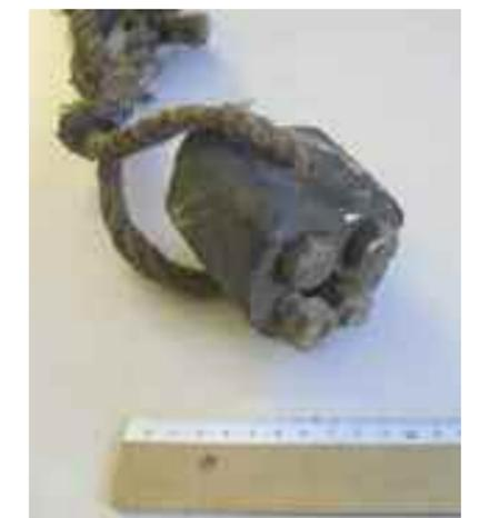
A solid piece of rubber gasket, with four steel bolts embedded to gain weight.
